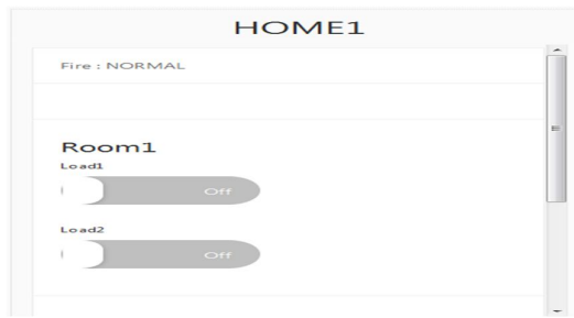
Fig. 8. The Web Page Of Home1 With Buttons And With Fire Status
